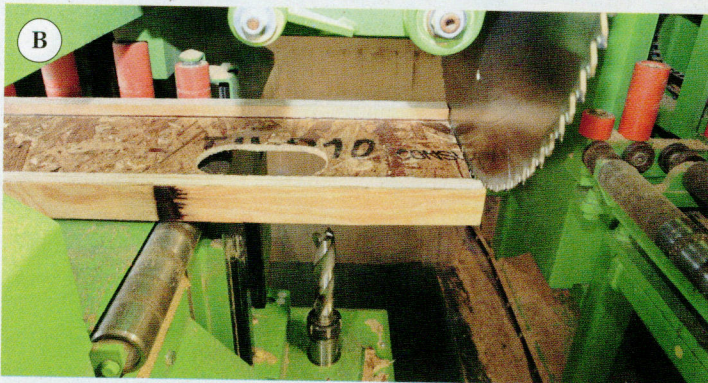
Figure 2. The engineered framing stock is cut with CNC equipment that can accurately trim I-joists and LVLs to length and cut bevels (A). The machine can also cut rafter-tail profiles and make hvac cutouts (B, C).
